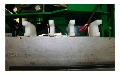
• Making sure that the two targets are just touching the back of the fingers, what we are looking for is a 2mm gap between the (TM79) driving rail and the driving band on the targets as per the picture below. Adjust the (TM79) driving rail in or out until you have this 2mm gap. Once you are happy with the adjustments tighten up the four fasternings and re check your work.
